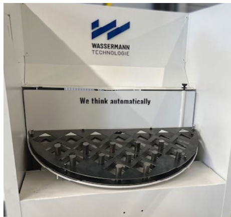
Configuration 2: Turntable: setup during the main processing time
