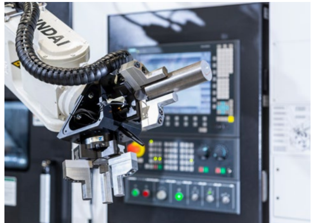
Double gripper for fast workpiece changes
