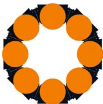
Level 1: 8 stations for workpiece dimension up to Ø 800 mm and workpiece height up to 350 mm
