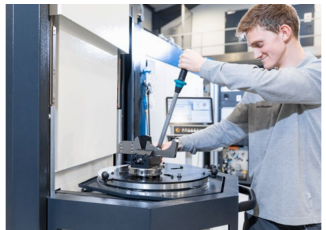
Ergonomic setup station for setup during primary processing, with mechanical interlock for maximum safety
