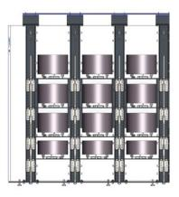
Division of the levels: flexible division of the transfer height from 250 to 500 mm, each with 0 550 mm
