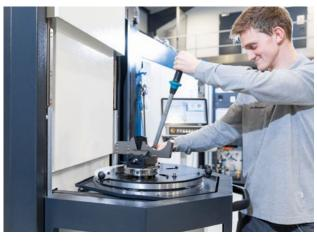
Ergonomic setup station for setup during primary processing, with mechanical interlock for maximum safety
