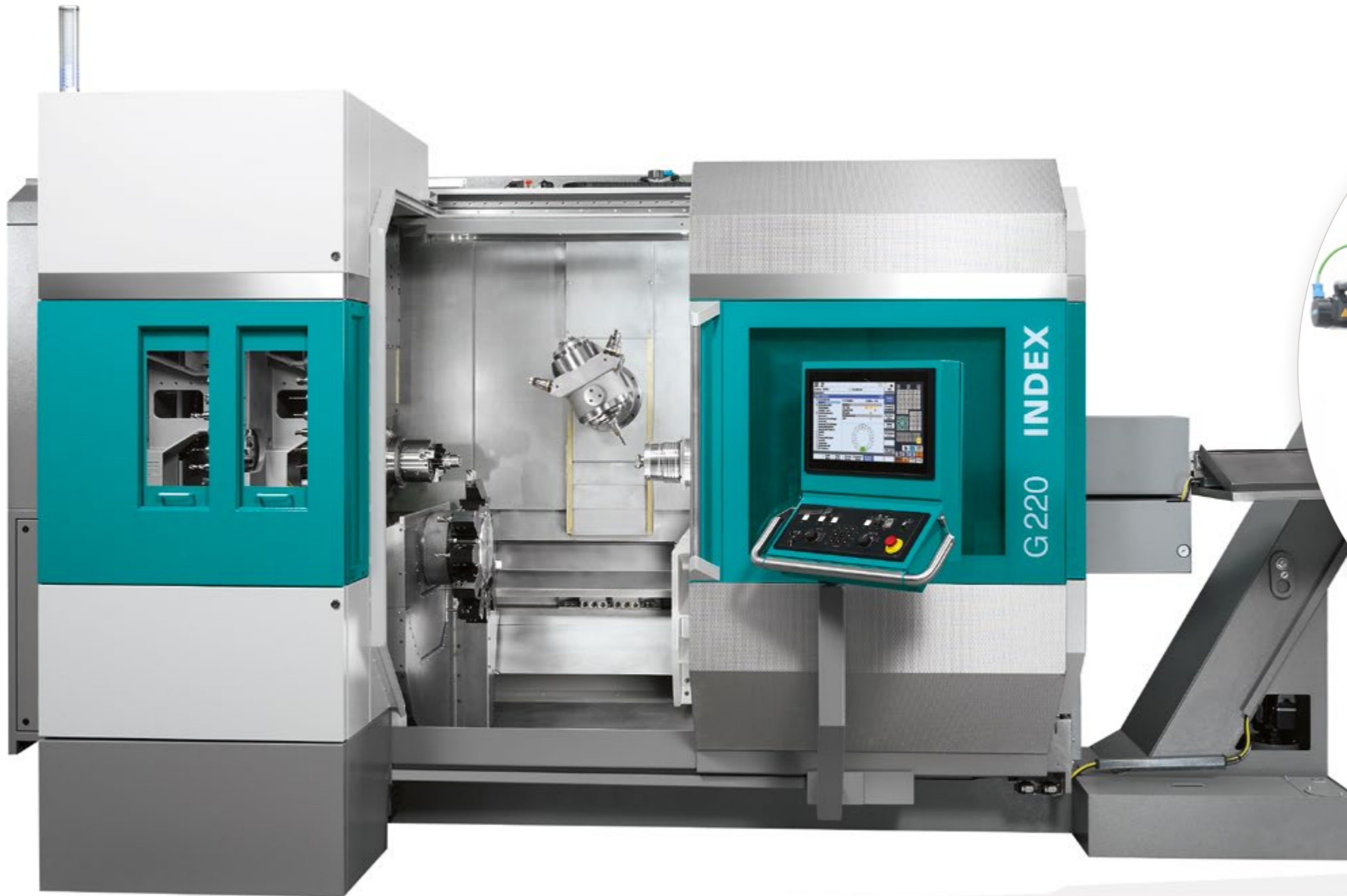
INDEX G220, equipped with a tool changing system from WASSERMANN TECHNOLOGY for 70 or 140 tools, change overtime 0,7 sec. (chip-to-chip time of 6 sec.)
