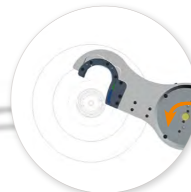
During the swivelling into place - the latch is retracted
