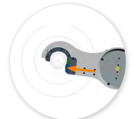
Swivelled into place and locked - Latch clamps the tool
